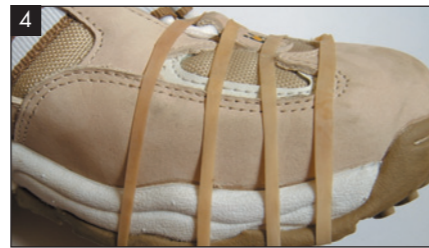
4. Hold surfaces together with elastic bands or clamps and allow glue to cure.
